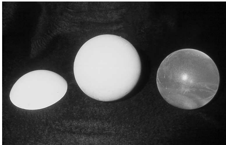
Fig. 1. Skin–skull–brain model. From left: Artificial scalp, hollow sphere of artificial bone (polyurethane), sphere of gelatin as a simulant of the brain.
